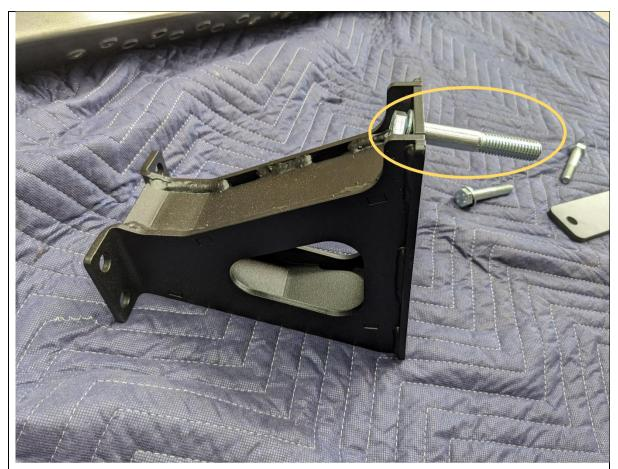
15. Prepare mid and rear mounts for fitting by threading through M12x90 Bolt through top hole.
