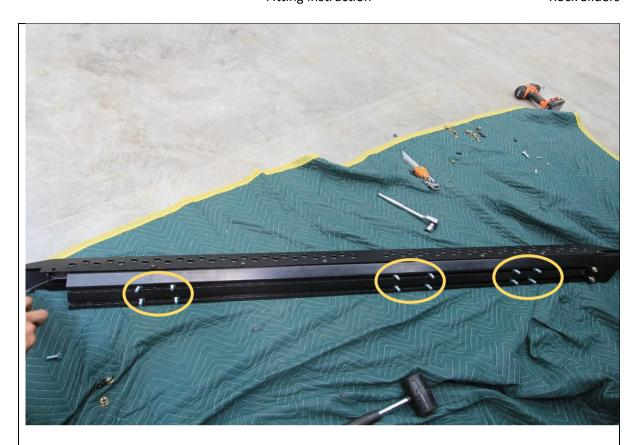
29. Slide the 12x M10x25 Hex bolts into the T slots on back side of extrusion. 6 bolts per slot.
